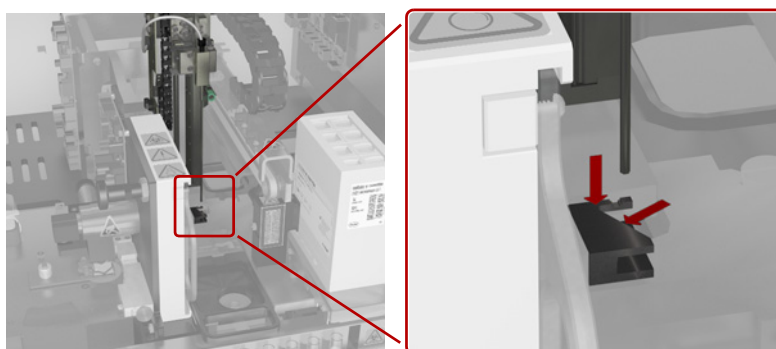
Figure 3-20 Probe bend detector on the test strip analyzer
